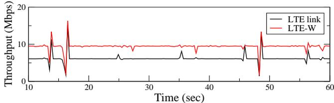
Fig. 3: Instantaneous throughput of total LTE-W and LTE link
