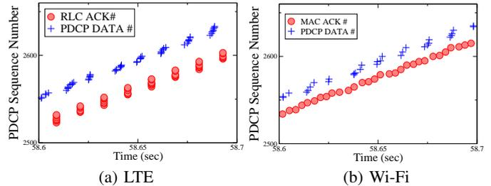
Fig. 4: Different ack transmission patterns: LTE and Wi-Fi.
