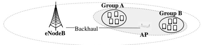
Fig. 5: Simulation node setup: 10 LTE-W UEs, Group A (5 UEs) and Group B (5 UEs)
