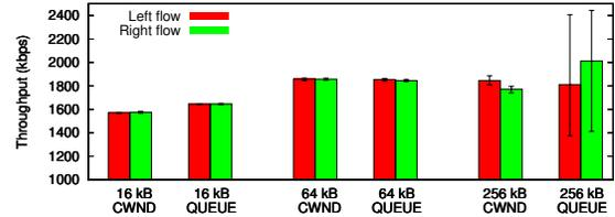
Fig. 10. Simulation. Effect of max physical queue size and  $CWND_{max}$  on TCP flows: Either bounded backlog by MAC or  $CWND_{max}$  by TCP can reduce TCP throughput since wireless channel is under-utilized due to increased back-off time with insufficient queued packets.
