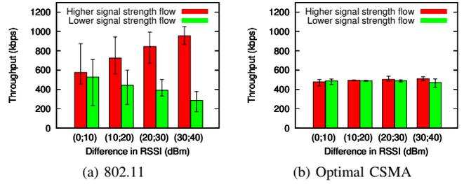
Fig. 8. Uplink flow throughput attained by two clients in CS range and associated with the same AP, in relation to the difference in RSSI measured from their signals at the receiver.
