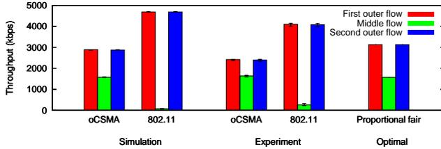
Fig. 6. Per-flow throughput attained by 802.11 and optimal CSMA in a topology with a flow-in-the-middle. To provide for comparison, the obtained results are presented together with the optimal throughput allocation for proportional fairness assuming an effective channel capacity of 4.7 Mbps. Simulation and experimental results were obtained using a 6 Mbps transmission rate.
