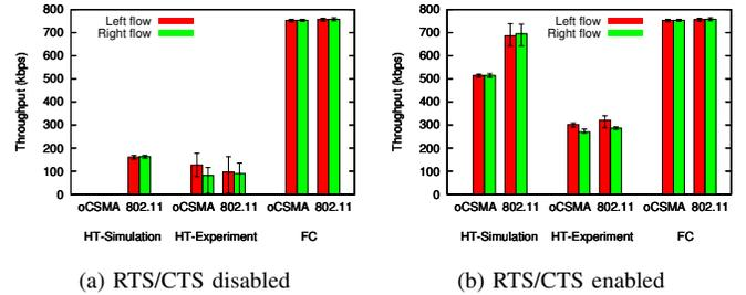
Fig. 4. Per-flow throughput attained by 802.11 and optimal CSMA in a topology with hidden terminals. To provide for comparison, experimental and simulation results are presented together with those obtained in a fully connected topology.
