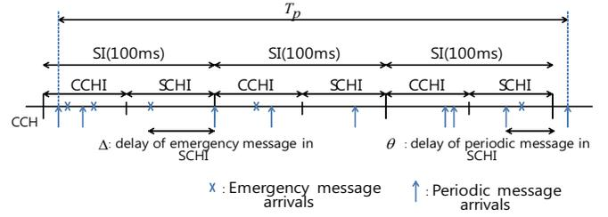
**Fig. 1:** Safety-related events occur on the alternating channel. (SI: Synchronization Interval, CCHI: Control Channel Interval, SCHI: Service Channel Interval.)
