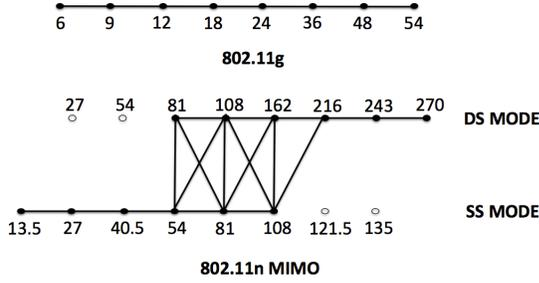
Fig. 1. Graphs  $G$  providing unimodality in 802.11g systems (above) and MIMO 802.11n systems (below). Rates are in Mbit/s. In 802.11n, two MIMO modes are considered, single-stream (SS) and double-stream (DS) modes.
