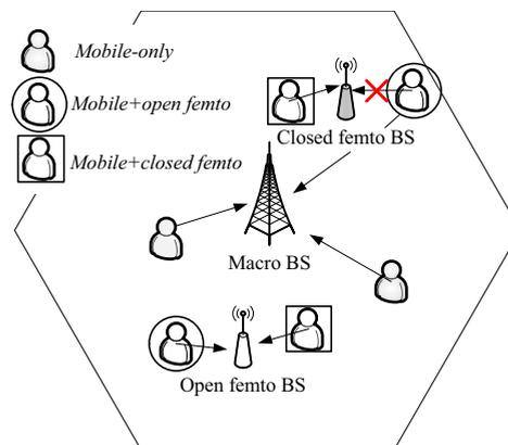
Fig. 1. Femtocell services: *mobile-only*, *mobile+open femto*, and *mobile+closed femto*
